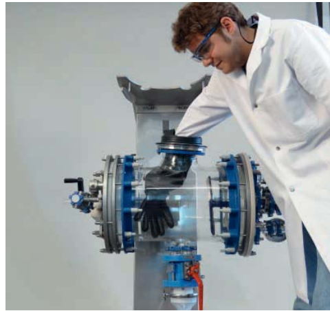
Removal of filter cake through containment system
