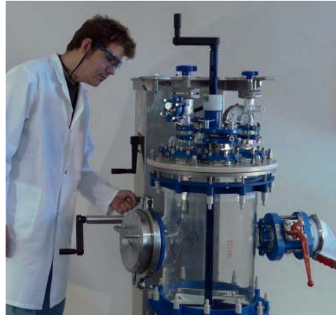
Simple lowering of filter vessel by hydraulic valve
